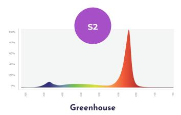
The \$2° spectrum is purpose-built for supplemental greenhouse lighting. It provides a comprehensive output spanning the entire PAR range (400-700nm), with additional energy concentrated in the red segment. Unlike typical "blurple" lights (which emit only blue and red wavelengths), S2© includes a substantial amount of green light. This design ensures that growers can inspect their plants comfortably, even when scouting for infestations, diseases, and nutritional concerns.
